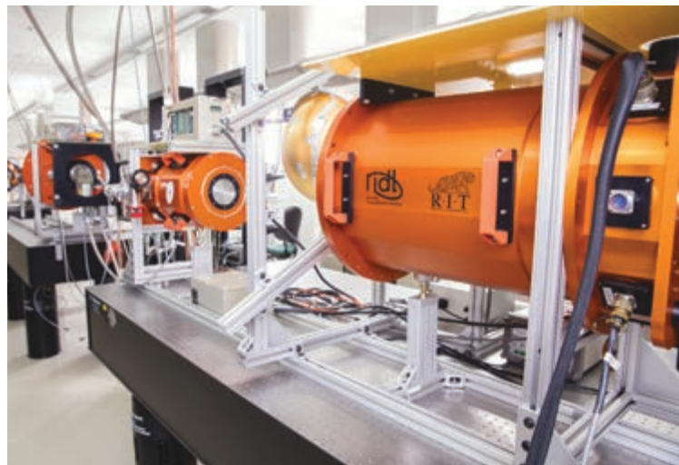
Imaging Detector Testbeds: These high-performance imaging detector testbeds in RIT's Center for Detectors give the FPI unique abilities to develop imaging devices for use in NASA missions.
