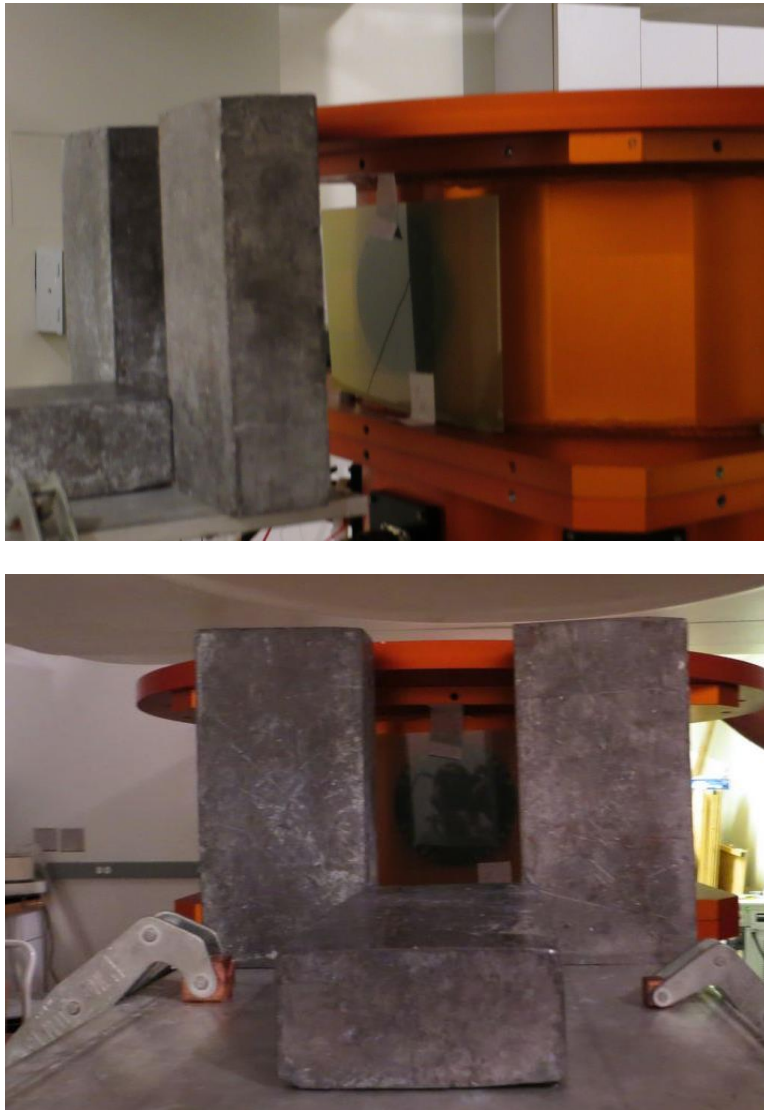
Figure 49 – This figures shows a close-up of the radiation testing setup around the dewar port. The top image shows a side view, and the bottom image shows the view as seen from the end of the radiation beam hardware (see Figure 47).
