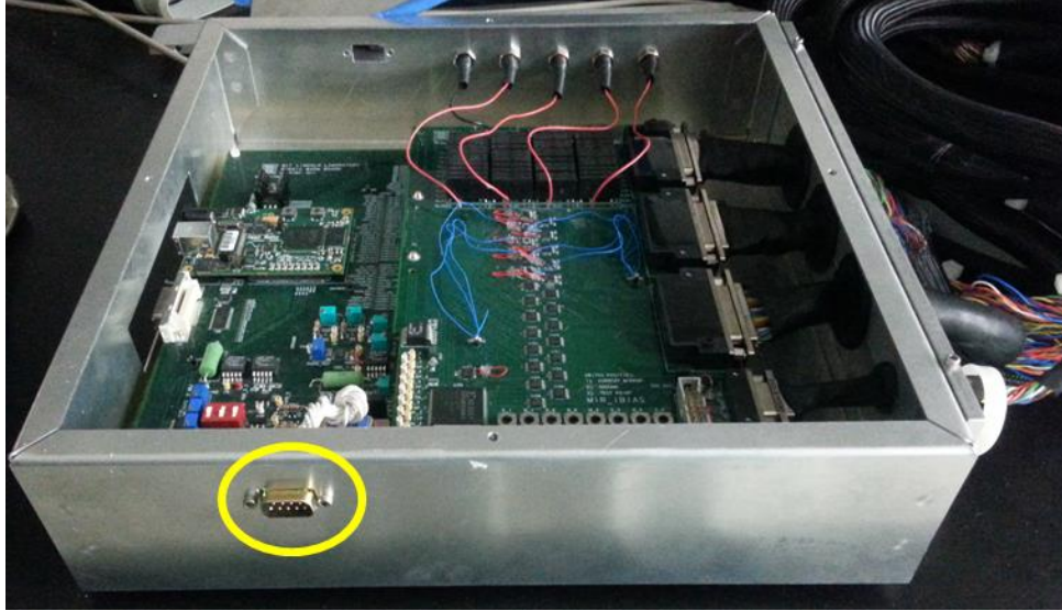
Figure 41 – The warm electronics housing with power supply connector (circled in yellow) is shown.
